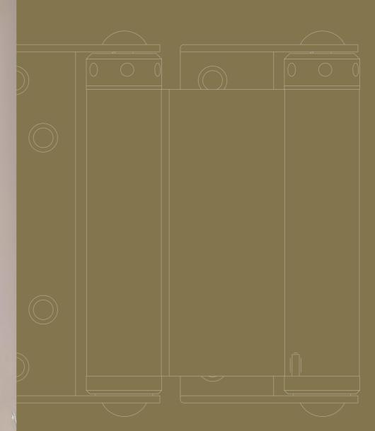
single 180/1 or double 180/2 With stainless steel pin and hardened steel spring. Includes key for tension adjustment
