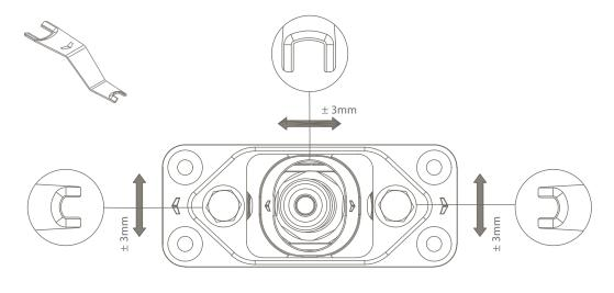
Upper pivot adjustable both in width and depth
